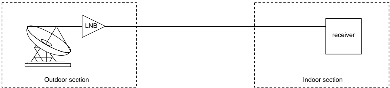
Figure 4: Simplified system diagram of a LNB receive system.
